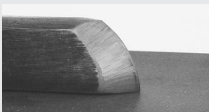
Skews have four surfaces to hone: two ground bevels and two side edges that define the short and long points (shown above).
