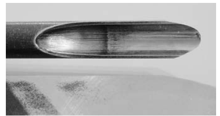
Milling marks in the flute of a gouge, above, and pits or milling marks on scrapers impact edge quality.
