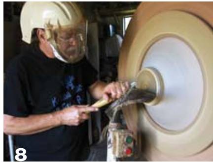
8 At his studio in Hawaii, AAW member Kelly Dunn details the bottom of a bowl with a homemade 36"-diameter Straka chuck on his bowl lathe.
